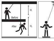
properly rated energy absorber. It is important to ensure that there is sufficient fall clearance below the user, before using a shock absorbing lanyard. If the weight of the wearer is 220 lbs. and the fall factor is two, we can calculate the fall clearance (which will be equal to the stopping distance H (2L+5.74 ft.) + an additional distance of 3.28 ft).
