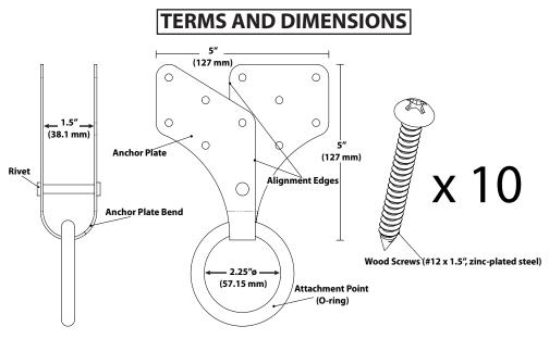
Minimum Breaking Strength (MBS): 1,800-lbf (8kN) Max Capacity: One person, 310-lbs (140 kg) Weight: 0.7 lbs. (.32 kg) Materials: Zinc-Plated Steel, Stainless Steel Regulatory Compliance: OSHA 1910.140, OSHA 1926.502
