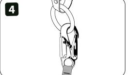
4. Connect personal arrest system (PFAS) to attachment point. PFAS must limit fall arrest forces to 900-lbf (4kN) or less.
