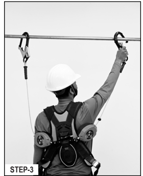
STEP-3 For lateral movement connect the second leg of the lanyard successive anchorage point.
