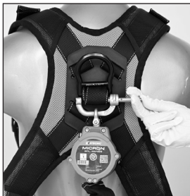
Slide Connector through loosened web straps placed below the Dorsal D-ring, then pull straps tight.
