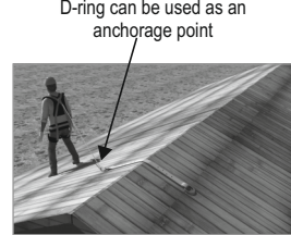
Fig. 3- Now the D-ring can be used as an anchorage point.
