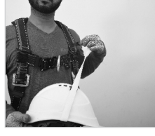
To attach clamp versions, take the clamp end of the lanyard and attach it to a shirt collar.
