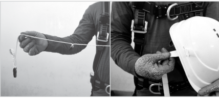
Take the free end of the lanyard and loop it through a captive hole on the Helmet accessory slot or suspension.
