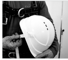
Take the connector end of the lanyard and pass it through the clamp.
