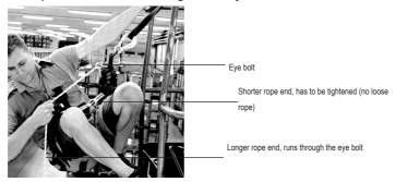
Using the eye bolts, you can control the descent speed or stop the descent. The longer, unloaded rope end runs through the eye bolts. If you hold on to the longer rope end, you can throttle the descent speed or stop the descent. If you don't use the eye bolts, the descent speed will be regulated automatically by two fly wheel brakes (speed ca. 0.8 m/sec)
