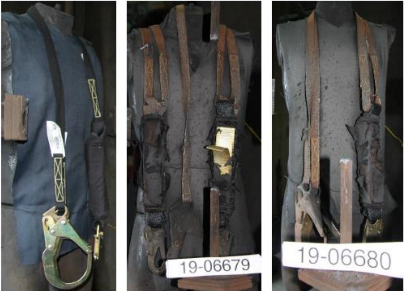
Figure 6-1: Sample before (left) after arc exposure tests 19-6679A (center) and 19-6680A (right).
