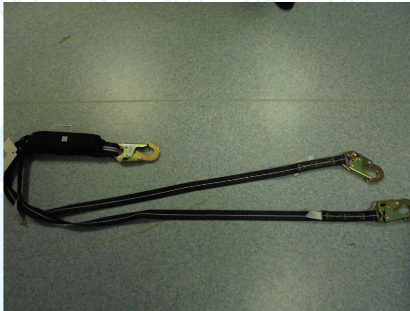
Figure 3 – Energy absorbing lanyard described as “FAP30198(WL)(6)”
