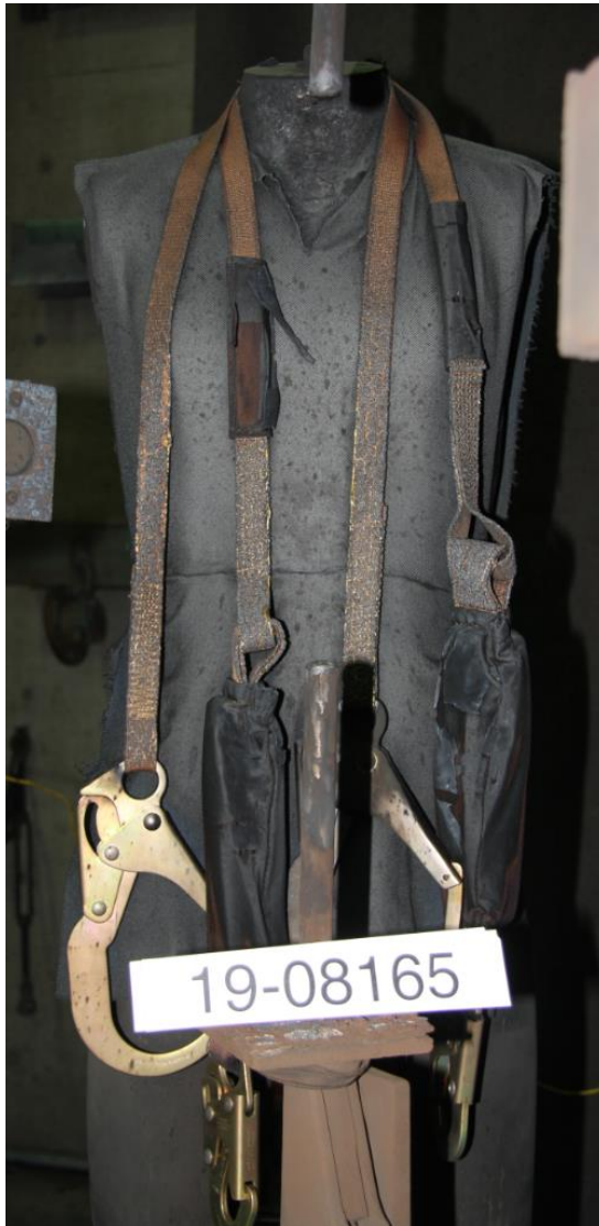
Figure 6-2: Sample after arc exposure test #19-8165 (A: left, B: right).
