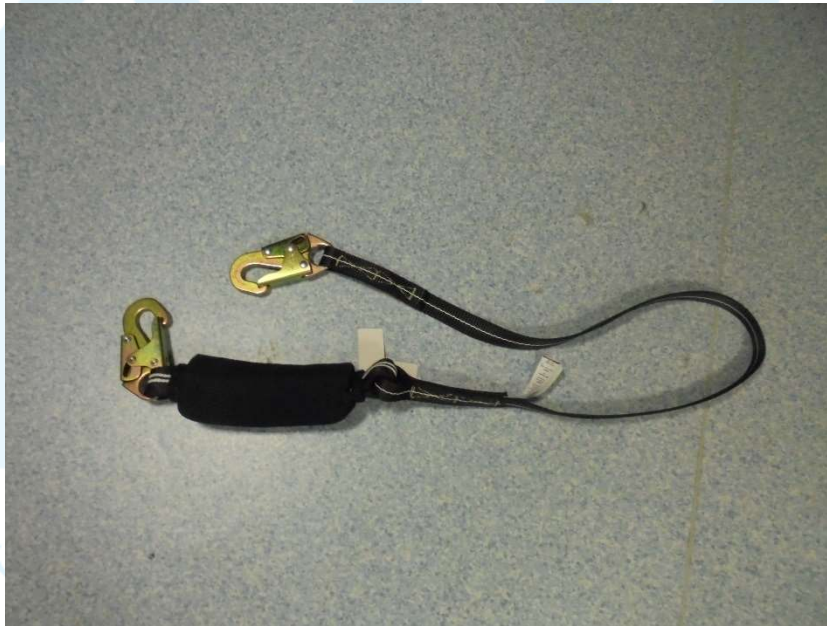
Figure 1 – Energy absorbing lanyard described as “FAP3118(WL)(6)”
