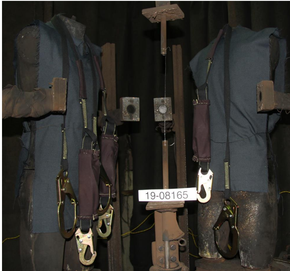
Figure 6-1: Sample before arc exposure test #19-8165 (A: left, B: right).
