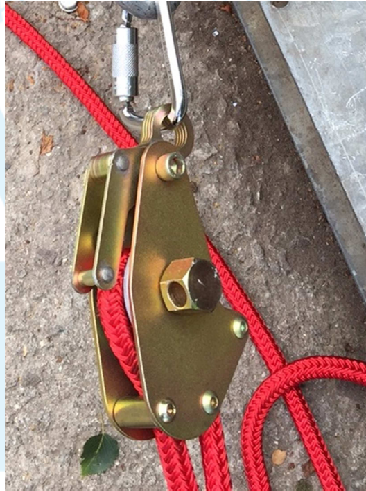
Figure 2 – Horizontal anchor line described as “PN 3002” Galvanised component
