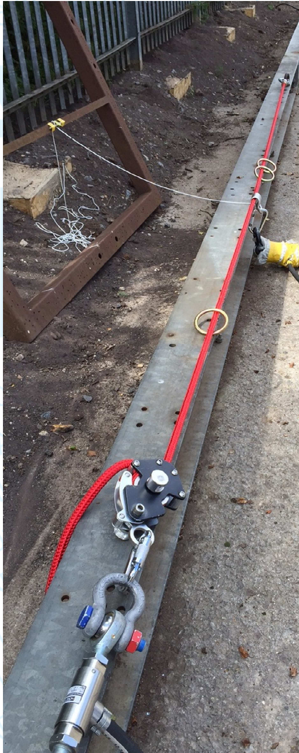
Figure 1 – Horizontal anchor line described as “PN 3001” (PN 3002 is identical but components are Galvanized)
