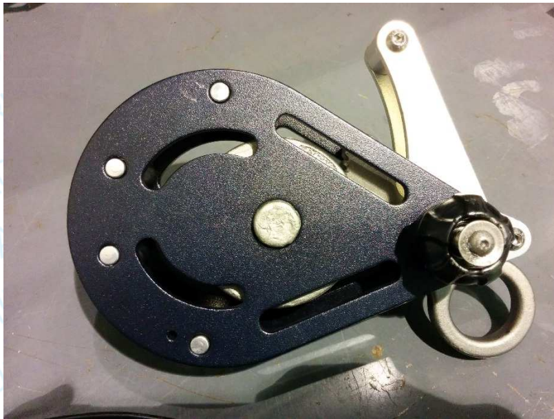
Figure 5 – New tensioner for PN 3001
