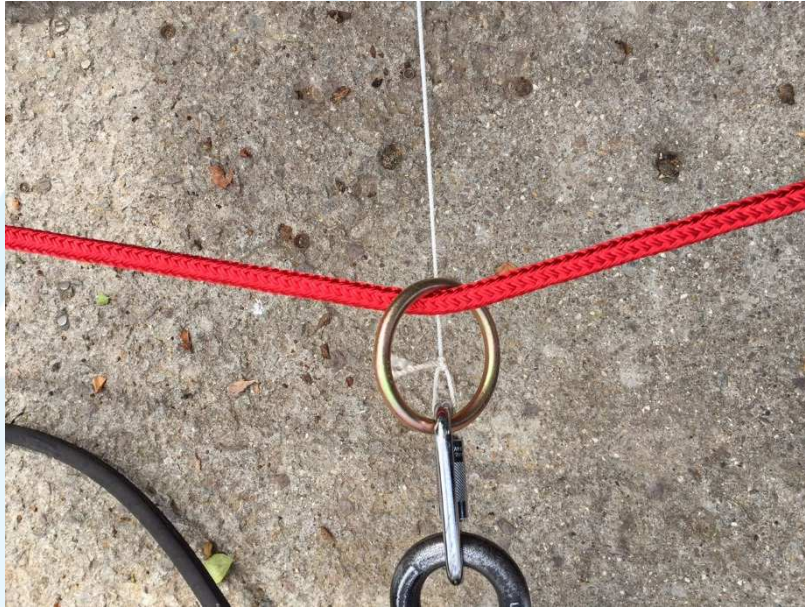
Figure 4 – D-ring anchorage attachment point
