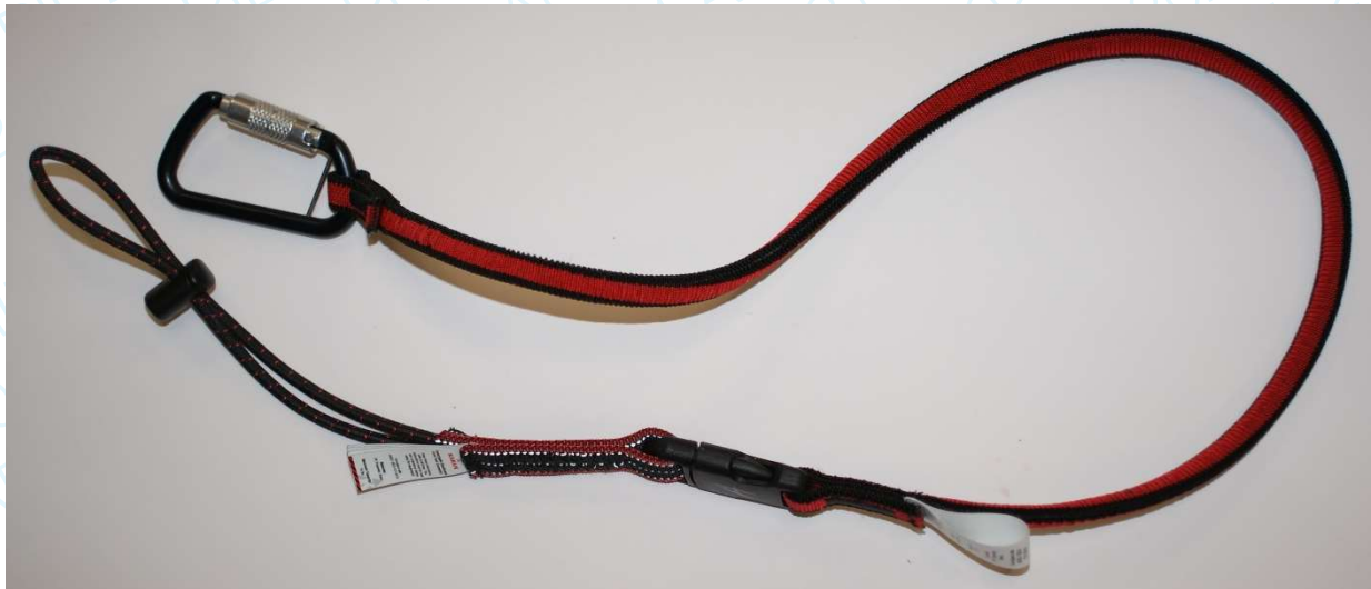
Figure 1 – Tool tether described as “DL100401” (made from the combination of components “DL100201” & “DL100400”)
