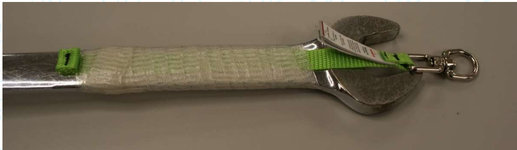
Figure 4 – Tool attachment described as " DL100351" fixed to the test mass using “DT700101”
