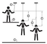
not exceed 2 ft. (0.6 m). Personal riding systems must be rigged so that there is no vertical free fall possible. Climbing systems must be rigged so that free fall is less than 18 inches (46 cm). Rescue systems must be rigged in such a way that there is no vertical free fall. Contact KStrong for any further information needed.
