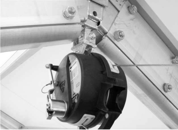
Simple Anchor Points at each end, with no intermediate supports
