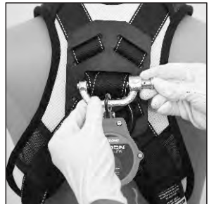
Push the pin inside the grooves of the connector to ensure locking.
