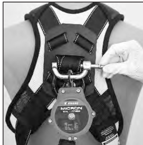
Slide Connector through loosened web straps placed below the D-ring, then pull straps tight.
