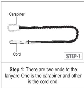
**Step 1:** There are two ends to the lanyard—One is the carabiner and other is the cord end.
