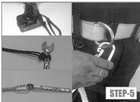
**Step 5:** Carabiner end—Hook carabiner on an appropriate attachment point. Attach on tool areas that are fully closed and/ or points where tool shape would prevent release.
