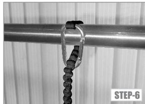
**Step 6:** Cinching carabiner is only advised on anchor points and belts and should only be done when tools are incapable of backing through.
