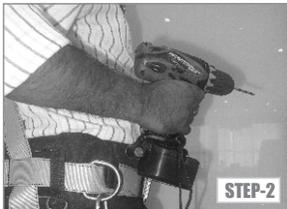
**Step 2:** One attached to the tool and other to the user/ fixed anchor point. Each end has a particular installation method.
