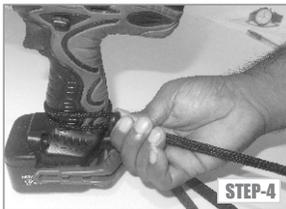
**Step 4:** The cord lock helps to keep the cord end cinched. Always make sure to secure the cord lock tightly down on the cinch and check periodically to maintain tightness.
