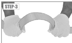
**Step 2:** Check the stitches on the harness. They should be intact, not cut or opened.
