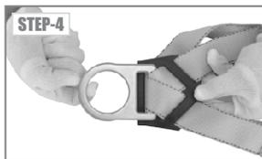
**Step 4:** Check the D-rings for sharp edges, distortion, cracks, breaks, and rough edges. Look out for any broken stitching of the D-ring attachments. Also, ensure the D-ring pivots freely.
