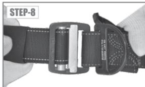
**Step 8:** Friction buckles should be inspected for distortion. The center and outer bars of the buckle should be straight. Carefully inspect the corners and attachment points at the center bar.
