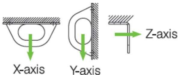
Tested to withstand load from all the 3-axes
