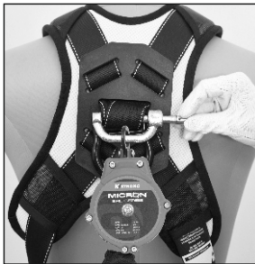
Slide Connector through loosened web straps placed below the D-ring, then pull straps tight.
