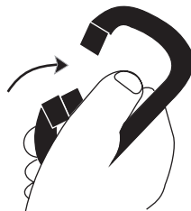
Open the gate by pressing it inside the body of the hook
