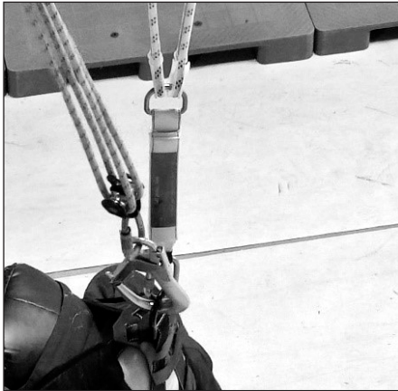
8. Once Scaffold Hook is attached to the casualty's attachment on the harness, pull and remove the pole from the Scaffold Hook.
