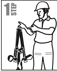
Step 1 : Hold the Harness by the Dorsal D-ring as shown in Step 1.
