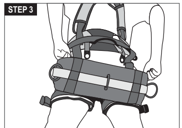
Position the seat under your upper thighs so that you can sit comfortably while suspended.
