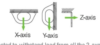
Tested to withstand load from all the 3-axes
