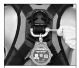
Open connector by pushing the locking lever and push button at the end simultaneously.
