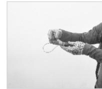
Place the tool connector on the handle of the tool in such a manner that the loop is free for tool attachment. Now tightly grip it with tool tape.
