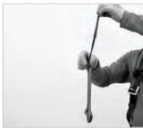
Tightly lock the knot with cord lock and the elastic tool attachment is ready to use.
