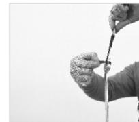
Now first pass the loop through the hole of the tool and then pass the D-ring end through the tool attachment loop forming a knot on the tool hole.
