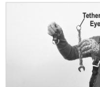
This tool attachment can be attached to lightweight tools that are provided with a tether eye (e.g. spanner).
