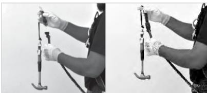
Join the male and female SR clamps to make one and the retro elastic tool attachment is ready for use.
