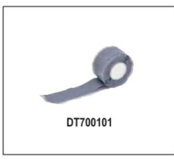
The tape layers will start to self-merge immediately with permanent adhesion within 24 hours. Repositioning is not recommended. Even though the silicone tape may be used under wet or oily conditions, an application on a clean, dry surface is recommended. The tape is not reusable, but additional tape layers can be added at any point in time.
