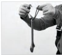
First pass the loop through the hole of the tool and then pass D-ring end through the tool attachment loop forming a knot on the tether eye.
