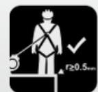
Block can be installed at foot level, in case installed near sharp edge having radius  $\geq 0.5\text{mm}$
