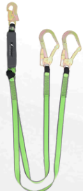
ELITE SHOCK ABSORBING LANYARD TWIN LEG 30MM WEBBING 1.8M C/W STEEL SNAP HOOK & STEEL SCAFFOLD HOOKS AT OTHER ENDS (AFL408612)
