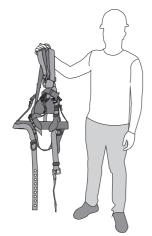
To don, hold the harness by the back D-Ring ensuring that the straps are not twisted.
