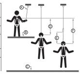
not exceed 2 ft. (0.6 m). Personal riding systems must be rigged so that there is no vertical free fall possible. Climbing systems must be rigged so that free fall is less than 18 inches (46 cm). Rescue systems must be rigged in such a way that there is no vertical free fall. Contact KStrong for any further information needed.
