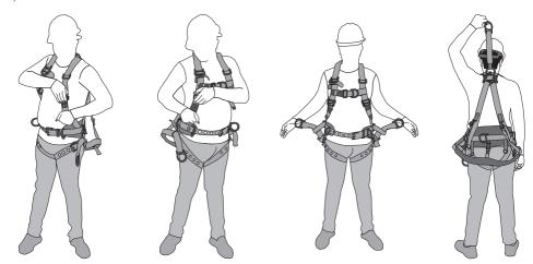
To check & adjust all the straps of the harness to your body adjustment, please check the all the attached points, they should be free to use. While in use, it is important to regularly check fastening and adjustment elements of the harness.
