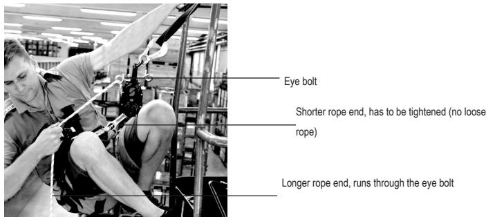
Using the eye bolts, you can control the descent speed or stop the descent. The longer, unloaded rope end runs through the eye bolts. If you hold on to the longer rope end, you can throttle the descent speed or stop the descent. If you don't use the eye bolts, the descent speed will be regulated automatically by two fly wheel brakes (speed ca. 0.8m/sec)
