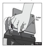
Lock the solid pin on mounting brackets using cotter pin.
