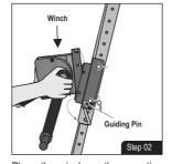
Place the winch on the mounting bracket of the tripod leg and insert the guiding pin into the slot.
