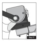
Locate the Extreme Stainless Davit arm that has pre-installed mounting bracket for installing the winch. Place the winch on the mounting bracket of the Extreme Stainless Davit arm and insert the guiding pin into the slot.
