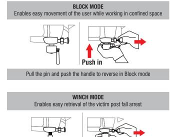
Pull the pin and handle to shift to Winch Mode
