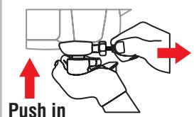
Pull the pin and push the handle to reverse in Block mode
