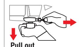
Pull the pin and handle to shift to Winch Mode
