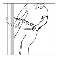
Use a suitable adjustable lanyard and attach it to the two side D-Rings by hooks or connectors while looping the lanyard to a vertical (preferably cylindrical) support as shown.
