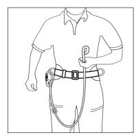
Tighten the belt on your waist by pulling the free end of the waist belt until the waist belt snugly fits the body without hindering free movement as shown.
