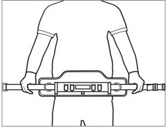
To achieve perfect fit of the work positioning belt, slide the waist belt by pulling from any side so that, the parachute buckle would lie in the centre of your stomach (below shows two arrows along which, the waist belt can be pulled out from the comfort pad to adjust as per the size of the wearer).
