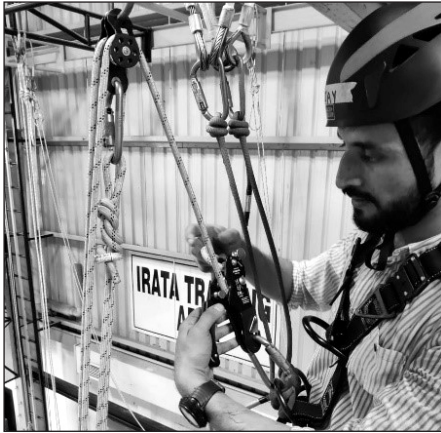
6. Connect the Descender to the rope and attach to the rescuer's chest D ring.
