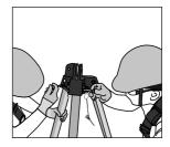
Lock & fix the Tripod by inserting the locking pins so that it stands firmly on the ground.
