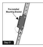
Locate the tripod leg that has preinstalled mounting bracket for installing the winch.
