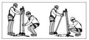
Stretch the three legs of the Tripod outwards so that they lie outside the periphery of the confined space into which entry is required.
