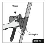
Place the winch on the mounting bracket of the tripod leg and insert the guiding pin into the slot.
