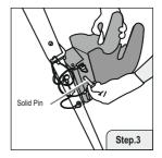
Place the retrieval mounting bracket on the lower mounting bracket pre-installed on the tripod leg and insert the guiding pin into the slot.
