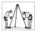
Now install & fix the Universal Brackets on the Tripod Legs to install winch & selfretracting lifeline, further.
