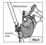
Insert retrieval block in bracket guided by aluminum guide provided on both side of retrieval.
