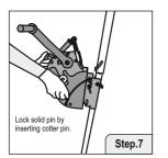
lock solid pin from other end by inserting cotter pin.
