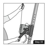
Pull out the handle of the winch outside and rotate it anti-clock wise to release the steel wire. Keep on releasing till you are able to release enough length such that it can pass over the pulleys of the tripod and get suspended vertically downwards.
