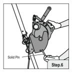
Lock the anchorage eye with bracket followed by solid pin.
