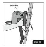
Use solid pin for locking the winch on preinstalled mounting bracket of tripod leg.
