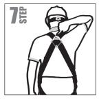
Use the back D-ring or the front as anchor point for fall arrest systems. To locate the anchor points on the harness, check for the "A" marking near them.
