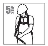
Close the buckles of the leg straps one by one as shown in Step 5.
