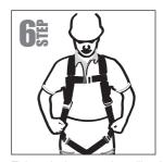
Tighten the leg straps by pulling the free ends of the straps until the harness fits perfectly to the body as shown in Step 6.
