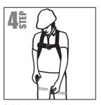
Pull the leg straps one by one around your thighs outwards to your front as shown in Step 4.
